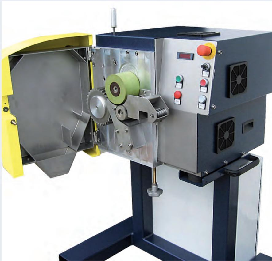
Good accessibility to the cutting area for cleaning and maintenance
