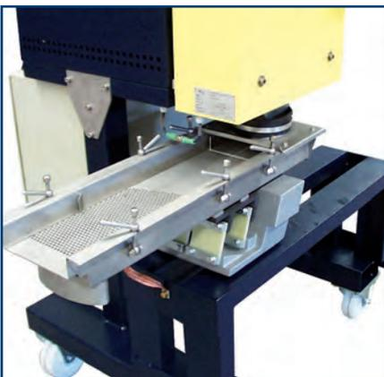
Classifier integrated into the machine frame
