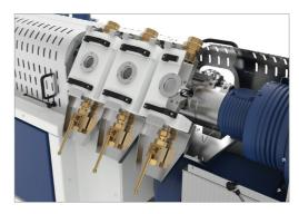
The efficient degassing provides the best possible pellet quality and increases the density up to 15%.
