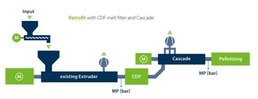
Existing filter can be replaced by the patented MAS filter Type CDF (**C**ontinuous **D**isc **F**ilter), which was developed especially for recycling applications to remove impurities such as wood, paper, non- melting plastics, rubber and similar contaminations from the melt. Due to the continuous operating principle the time- and labour-intensive exchange of mesh filters can be reduced to a minimum.
