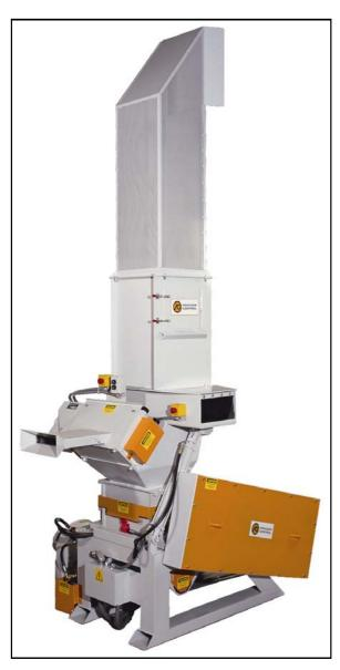
The GF Series: film scrap grinder for use with asr® systems to recycle edge trim, roll scrap, and loose scrap (pictured above is a GFCN30 with optional roll feeder, hydraulic lift, and AEN air eliminator).
